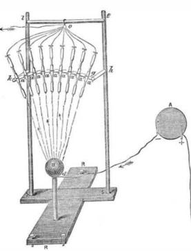
A is an electrical machine, the negative pole being connected with a copper sphere and the positive with the earth. S S' aro of ebonite, as well as R R dd, so that B is quite isolated as the earth in the spac. B is surrounded by the atmosphere. a' a' a' a' a' are a series of Geissler tubes with copper ends above and below. All the upper ends are connected with a wire which goes to the earth, consequently a current runs in the direction of the arrows through the air,
