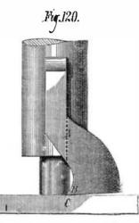
line, A, or fulcrum from which the springing takes place; hence, when the tool springs, it will recede from the work, C. To avoid springing and for very large holes, the cutter may be a short tool, held by a stout crossbar carried by the stock; but in any event the cutter should be made as shown above.
