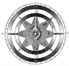
This compass is said to be much more sensitive than the needle, to be less affected by rolling of the ship, and to be much less sluggish than the liquid compass. These facts were adduced by recent French naval tests of the instrument in comparison with compasses of the usual construction.
