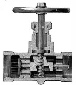
stop valve recently invented by Mr. Whitton, and introduced by Messrs. Low and Duff, of Dundee, Scotland. Its chief characteristic is its powerful closing and opening movement, obtained by a combination of the screw and the wedge. This gives it a ready control over the supply of steam or water under great pressure, and especially adapts it for use as a throttle for a locomotive or as a water hydrant valve.
