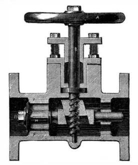
adjusted by studs. The seat of the valve, being put in separately, can be easily repaired. The bottom of the screwed spindle is also recessed into the bottom of the valve, giving lateral support to the spindle.
