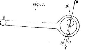
the joint of the slide valve spindle and eccentric rod end, B, the line representing the throw of the eccentric, and show ing the position in which the eccentric requires to be set in the case of the lesser valve travel, C, a line representing the throw line of the eccentric as it is when the eccentric is made to suit the increased valve travel, and the dotted line, D, a
