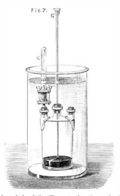
of air through the shell. 'The test tube, K, remains filled with water. We have thus the proof that a dry shell, or even one recently wet, is totally impermeable to gas.
