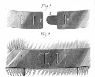
vice, which is both simple and ingenious, may be entirely made by machinery and placed in the cooper's hands complete in itself, no hammering being necessary to put it together for driving on the barrel. It requires no rivets; and hence the labor of making holes and of securing such fastenings is obviated, thus saving time and expense. Fig. 1
