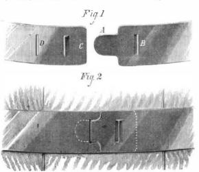
cutting of said slot at three sides being bent to the rear. The opposite end has also a slot, C, similar to B, the piece being, however, turned to the front, and another opening, D, from the interior of which the metal is altogether removed. In locking the ends the tongue, A, enters the opening, D, as in-
