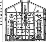
late government architect, has patented an improvement in the construction of prisons, shown herewith, which consists in combining two ranges of cells, C C, with a partitioned or double corridor, G. The heating apparatus is below, and the arrows show the courses of the the air, which passes through each cell, and
