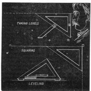
The hypothenuse of the triangle is conveniently made  $7\frac{1}{2}$ inches long, the other sides being  $4\frac{1}{2}$  and 6 inches, respectively. A plummet indicates the correct position of the instrument. It can readily be adapted for leveling horizontal surfaces, by adding a spirit level, as shown in the engraving. H. C. NAYLOR.
