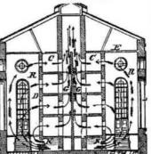
Mr. Alfred B. Mullett, late government architect, has patented an improvement in the construction of prisons, shown herewith, which consists in combining two ranges of cells, C C, with a partitioned or double corridor, G. The heating apparatus is below, and the arrows show the courses of the the air, which passes through each cell, and
