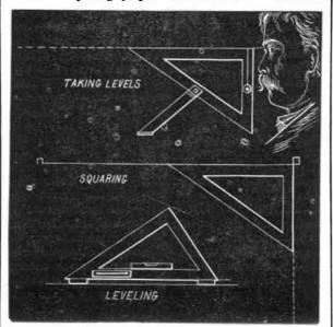
The hypothenuse of the triangle is conveniently made 7½ inches long, the other sides being 4½ and 6 inches, respectively. A plummet indicates the correct position of the instrument. It can readily be adapted for leveling horizontal surfaces, by adding a spirit level, as shown in the engraving.
