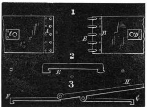
In Fig. 1. A. B. C. and D are pieces of No. 16 sheet iron. riveted to the ends of the belt; EE are hooks, shown in the natural size in Fig. 2, riveted to B. After the belt is laid over the pulleys, the hooks, F and G, of the lever, shown in Fig. 3, are placed in the holes at C and D. Now the two ends of the belt are drawn together by the lever, H; and the hooks, E, are put in their places at A. Then the lever is taken out, leaving the joint finished.
