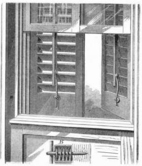
which the wheel and tyre serve as a balance wheel. It is latter outward, and so bind the wire between the cap and staple. A sectional view of this arrangement is shown at B. The blind slats may be set in any position, and are held by the wire.
