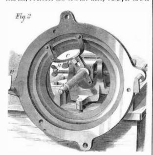
The feed nut is closed over a projection on the end of the block in which the shaft runs; so that when placed on an angle, there is no tendency to cross the thread of the screw. The irregular motion, which is inseparable from a machine which makes a taper hole, occurs, it is stated, only at the point where the arm touches the feed nut, and is simply a sliding back and forth of the former as the wheel is turned.
