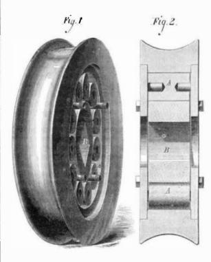
friction rollers arranged within the disk. This distributes the strain over a larger surface, rendering the operation easier, and subjecting the parts to much less wear than is the case in the ordinary arrangement of a small pin, which may readily fall in between two of the rollers and so crush the same.
