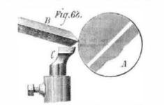
hand rest (the point being used to cut, as shown in Fig. 68, A being the work, B, the graver, and C, the lathe rest), it turns very true and cuts easily and freely. This, therefore, is the position in which it is held to rough out the work.
