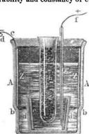
the engraving, of a glass vessel, A A, 8 inches high and 5 inches wide, in the bottom of which is placed a small glass vessel, d d, of half the dimensions of the larger glass, cemented in with rosin. A zinc disk, Z Z, which is supported upon a ledge of the outside vessel, surrounds the smaller glass. The inside wall of the smaller glass, dd, is covered by a sheet of copper, e, on the lower end of which an insulated copper wire, g, is riveted. The mouth of the
