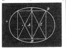
square, bisect it, and draw diagonals in the halves of the square. Describe the oval with the compass, using A, C, B, and E as centers.
