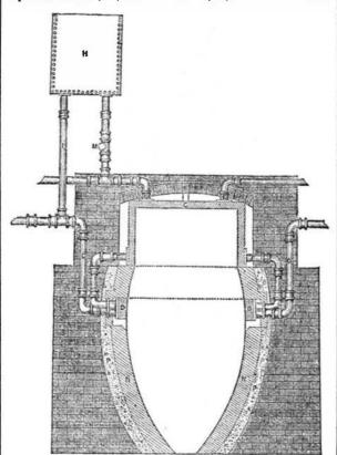
ty valve to the whole apparatus, and is therefore indispensable. The condensed water from the cistern, H, is returned to the annular boiler, D, through the perpendicular pipe, I; M is a valve in the flow pipe to the expansion cistern, H; and the pipes, E, communicate with all the premises to be warmed, and through valve, M, with compensating cistern, H. A blow-off cock for the annular boiler is necessary.
