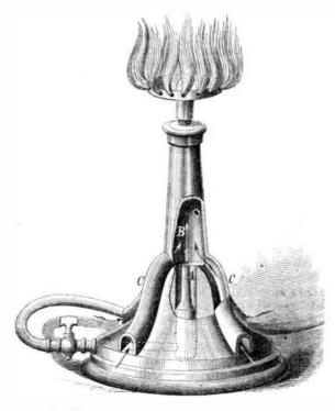
cate with the chamber. The burner, the tube of which leads from the compartment last mentioned, is of any desired form.
