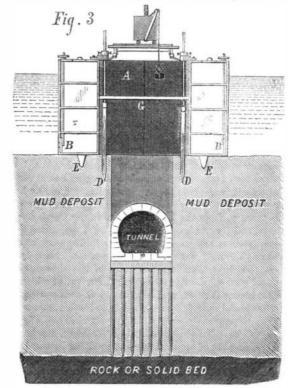
cipal feature of the invention is the system of place piles which surround the interior sides, and which may be forced down below the bottom of the dam and into the mud for a
