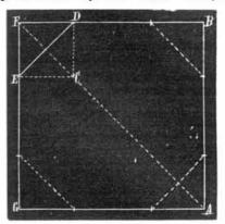
CEFD, and line from D to E will be one side of the octagon. Proceed in the same manner in the other angles of the square A B FG. Is this a correct method? A. Yes.
