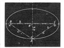
Take one half the length (2inches) and measure from A, 2 inches, striking the line of the length at Band C; then set pins at A.B.and C. tle yourstring.b. around them; then pull up pins at a', and use the pencil as you describe.
