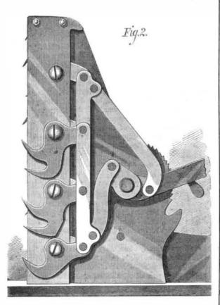
18 inches may be sawn up from the first dogging, without rolling the log, as two teeth must enter the lumber, and these are sufficient to hold it securely. When the surface towards the dogs is wide, five or more teeth can be driven in, at the will of the operator.
