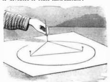
To make an oval, tie together the ends of a thread or string. Two pins arranged within the loop, as shown, gov ern the size of the oval, which is marked upon the paper by means of a pencil, carried against one side of the loop as in dicated. The dimensions of the oval may be made larger or smaller, as desired, by enlarging or diminishing the size of the loop. Elliptical garden paths, flower beds, etc., may be accurately laid out in this way.
