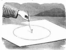
To describe a circle, attach one end of the cord to the cen ter pin, and place the pencil in a loop at the other end. Then sweep the pencil around.
