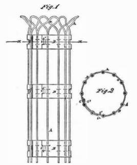
ormed in said straps, B, near their other ends, as shown in Figs. 1 and 2. In the straps, B, at their square ends, and at a little distance from their tongued ends, are formed holes b3, Fig. 2, in such positions as to coincide with each other when the ends are overlapped, to receive a short bolt, C, which is secured in place by a nut screwed upon it. The outer arm of the last wire loop at each end of the straps, B, overlaps the last arm of the loop at the other ends of the
