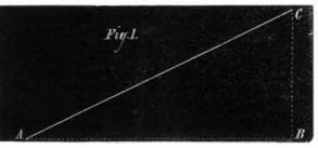
lix, which can be traced on the cylinder by using the edge, A C, of the paper as a guide. If the helix is to be constructed for only a portion of a revolution, make A C equal to that fraction of the circumference, and B C equal to that fraction of the pitch. Similarly, if the helix is to make several revolutions, A B must be the length of the circumference of the cylinder multiplied by that number of revolutions, and B C, the pitch multiplied by the same number.
