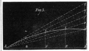
B D is equal to half the sum of the initial and final puch. Divide C D and A B, each into the same number of equal parts, and mark the points of intersection of lines drawn from the divisions of C D, to A, with the perpendiculars erected at the corresponding points of A B. A curve, D123A, drawn through these points and D and A, will be the guide, by means of which the required helix can be traced upon the given cylinder.
