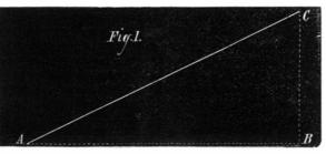
lix, which can be traced on the cylinder by using the edge A C, of the paper as a guide. If the helix is to be constructed for only a portion of a revolution, make  $\Lambda$  C equal to that fraction of the circumference, and B C equal to that fraction of the pitch. Similarly, if the helix is to make several revolutions, A B must be the length of the circumference of the cylinder multiplied by that number of revolutions, and BC, the pitch multiplied by the same number.
