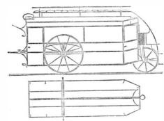
wider and lighter body to be used than in an ordinary omnibus, the total weight of which ranges from 20 to 24 cwt. for 26 passengers; for the same number of passengers, a threewheeled omnibus might be made to weigh from 14 to 16 cwt.
