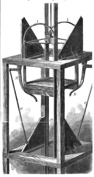
The hatch covers are separated diagonally and are lifted as the car ascends by the curved upper portion, A, of the latter. As the car continues its upward course, the covers are kept raised by means of the bell crank levers, B, connected thereto by rods, C, which levers press against the sides of the car and ease the fall of the doors. In descend- by a warm stove while drawing in the fish.
