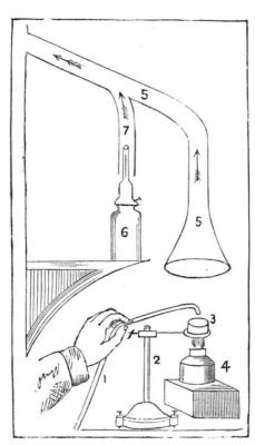
No. 1, a glass tube connecting the gas bag with burners No. 2, an iron stand to hold the small crucible. No. 3, a crucible. No. 4, a small alcohol lamp to ignite the sulphur. No. 5, a funnel to receive the product of combustion. No. 6, a petroleum lamp employed to establish a current of air in the chimney. No. 7, a shaft connected with the chimney, in which the current of air is formed by means of gas or a
