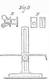
the block complete, the scriber being a simple piece of round steel wire. The dotted line on the foot is the distance to which the foot is hollowed out to make it stand firm. Fig. E is the bolt and nut; the bolt has a flat side filed on each side of it to fit it to the slot in the scri bing block stem, so that the bolt cannot turn when it is being tightened. Fig. F is a face and edge view of the piece or clamp for the scriber which passes through the hole in the elot.
