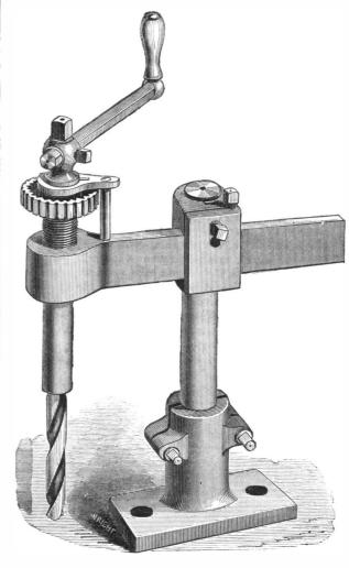
A charge of spindle can be made almost instantly to suit drills of different shanks, and if desired a hand feed can be used. The arrangement for holding the standards is such that, with any reasonable degree of care, it will not be marred.
