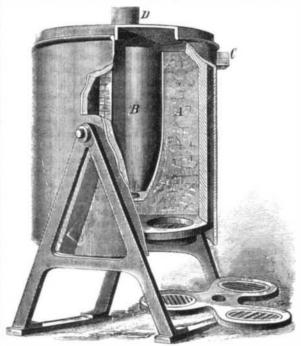
ing process. A suitable lever connects with one of the bearings for convenience in tilting the furnace.
