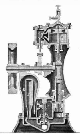
By the unscrewing of a single nut and the withdrawal of a key, which is inserted by hand, the discharge valve and seat may be taken out, thus giving access to the suction valves underneath. The key above mentioned is not driven in, but its end rests against the hand hole cover, so that it cannot by the ship. We have received a letter from Captain Blakework out of place.
