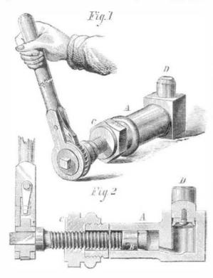
at the circumference, for expanding and closing tightly the more the pressure is increased, and is connected by a universal or similar joint to its screw bolt. The screw nut, C, is affixed at the end of the tube, A, and through it the bolt passes, terminating in a square end, to which the ratchet wrench is applied.
