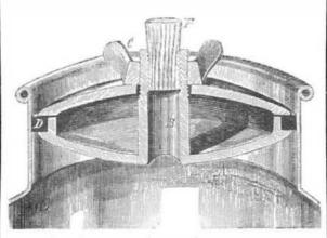
ward against the inner surface of the can, making a rigid airtight joint. The plug, E, is subsequently screwed down into the milk, forcing it into every interstice of the can, and so preventing its shaking about during carriage. Patented | from that containing other fats. February 24, 1874.
