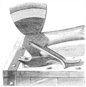
on pressing down on the latter, two dogs, A, pivoted, as shown, to the hatchet, enter the wood surface and thereby force the claw under the head of the nail. By further pressure the handle becomes a lever with the fulcrum formed by the projecting piece, B, so that the claw is carried straight apward, thus pulling the nail in that direction.
