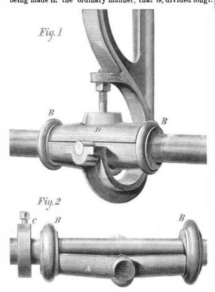
tudinally, and the halves united by bolts) is constructed of two portions of unequal size. The idea of the inventor is to produce a bearing, the ends of which, in taking against the usual collars or rings, secured to the shaft to prevent end motion of the box, shall not cause the unequal wear of the collars and the consequent disagreeable noise.
