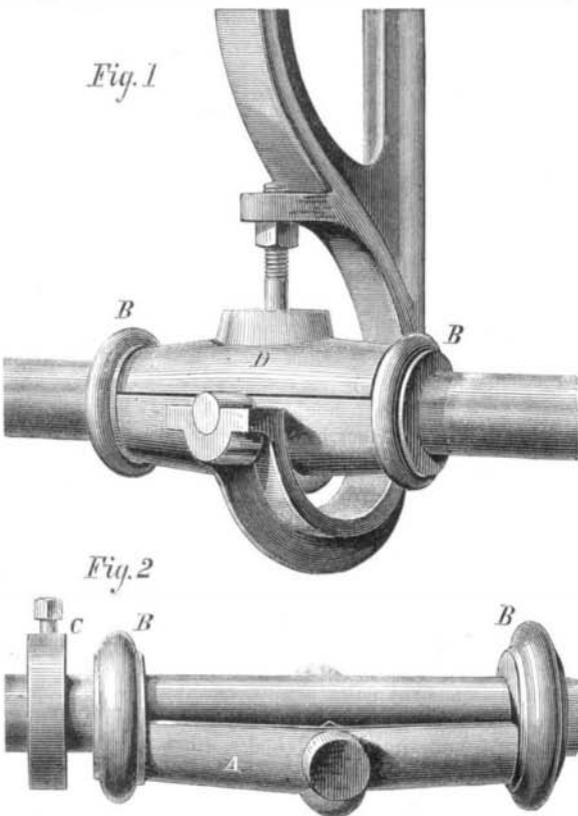
tudinally, and the halves united by bolts) is constructed of two portions of unequal size. The idea of the inventor is to produce a bearing, the ends of which, in taking against the usual collars or rings, secured to the shaft to prevent end motion of the box, shall not cause the unequal wear of the collars and the consequent disagreeable noise.
