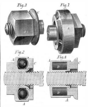
In Figs. 3 and 4, small cylinders of rubber are substituted for the balls, D, and the washer enters directly between the flanges. The tubular end of the nut is upset on the hole of the washer, in order to prevent separation of parts. The device appears simple and practical, and doubtless will meet with extended application upon railroads.
