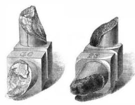
No. 71 is a piece of tool steel, having a strength twice as great as the best of iron, great elasticity, but a ductility only a fraction of that of good iron, excellent, in consequence of its strength and hardness, for tools and for resisting steady strain, but not so well adapted as steel of lower grade, or even as the better grades of iron, to meet shocks. Its jagged fracture and its fine even grain are evidence of the splendid quality of the metal and the perfect homogeneity of struc-
