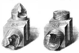
ture, which distinguish it from the fiberous wrought irons. The shear steels and the softer grades of tool steel usually exhibit an appearance very similar to 68, but are apt to crack along the side and through the neck, as is illustrated in No.
