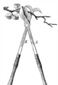
handles past each other without changing the hand, when the other edge of the blade acts with the hook precisely as before. In this way, the inventor says, a person may remain in one position and prune a tree nearly all around.
