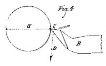
a being the shaft as before, B the tool, and C the shaving, the dotted line D is the direction of the strain put upon the tool by the shaving, which has but very little, if any, tendency to spring the tool into its cut.
