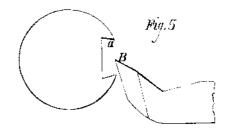
4, not because it is the best tool to cut the metal, but be cause it is the least liable to spring into its cut.
