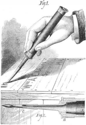
traced, as the flow is regulated by the pressure of the hand upon the compressible tube.
