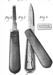
spring catch, A, in the position in Fig. 2. In both cover and box, just outside the pivot, is formed a jaw, so that, when the parts are closed together, a dovetail socket is made, which receives the correspondingly shaped ends of the tools. Fig. together. Mr. John Griffen writes to correct the impression 3 is a transverse section of this portion, and shows the shape of the jaws. This invention was patented February 11, 1873,
