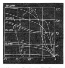
graphic machine. It will be seen that they are so formed that each point of the curve is so situated that its hight above the base line (that is its ordinate, as it is called), measures the force which strains the piece to a degree which is proportional to the distance of the point from the right hand border of the diagram, that is to say, the latter distance is the abscissa of the given point.
