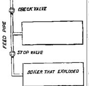
would go into that boiler in which the pressure was least. The whole system of connections in these boilers, both in steam and water spaces, appears to have been very faulty ; and in addition, much testimony was taken to the effect that the boiler was not well built, so it does not seem difficult to find reasons for this explosion.
