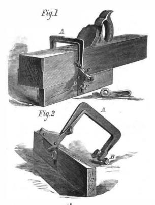
By fixing the plane (with guide attached) in the vise, small work can, it is stated, be squared or beveled without the annoyance of frequently picking up and laying down a heavy plane, try square, or bevel, several times for each piece, and the trouble of fastening each piece in the vise. This work can be done perfectly, with the attachment, where the light would be insufficient for the ordinary mode of operation.
