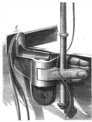
dragging upon them by the horse only wedges the clutch tighter. The apparatus is made of malleable iron, is quite strong and durable, and, it is claimed, cannot become out of order.
