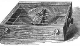
longitudinal sides higher than its transverse ones, in order to receive a glass cover. The center of the latter is thickened into lenticular form at A, in order to afford the necessary magnifying power. B is a small platform, which is
