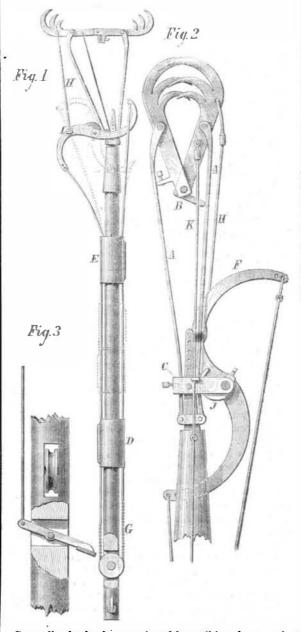
Generally the hooks are tripped by striking them against the back of the fish at the joint; but as, in case of striking a stone or other hard substance, the points might be injured, a wire, K, is connected to one of the prongs near the joint, and extends up to a small trip lever shown in Fig. 3. This lever, worked by the finger, pulls the joint back, and so trips
