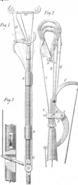
Generally the hooks are tripped by striking them against the back of the fish at the joint; but as, in case of striking a stone or other hard substance, the points might be injured, a wire, K, is connected to one of the prongs near the joint, and extends up to a small trip lever shown in Fig. 3. This lever, worked by the finger, pulls the joint back, and so trips the hooks.
