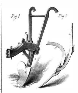
cility and celerity, simply by turning a hand screw on top of the beam. It is claimed that there is nothing about the device to wear out, give way, get lost or misplaced, or become out of order. No single portion is detached at any time, and the operator can tighten the fastening apparatus while plow ing with perfect ease
