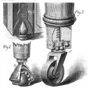
Fig. 2 shows the invention more especially adapted to protecting trunk casters from injury. In this case the cup in which the ball revolves is secured in a cavity formed in the bottom of the trunk by means of tongues, E, struck up from the sheet metal lining of said cavity. Thus arranged, it is stated, the caster will sustain severe concussions and great pressure.
