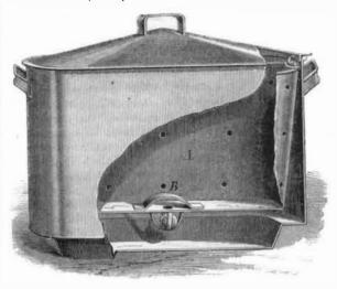
is a ball held in wires or similar contrivances by which its movement is limited. It will be noticed that the inner vessel, A, fits into the boiler steam tight, and that it may be readily lifted in or out, for cleansing or other purposes, by the handles, one of which is shown at C.
