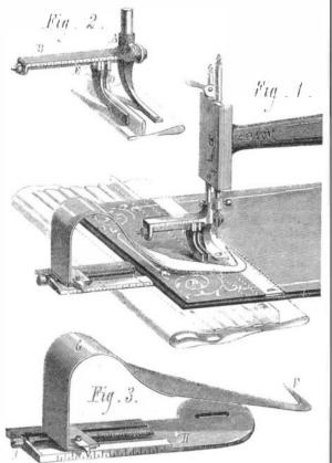
in a dovetail on the index plate, H, engaging with the temper screw, I. The slot represented in the shank of the index plate serves to secure it to the platform of the machine in the position shown in Fig. 1.
