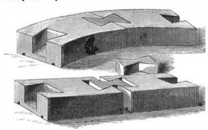
The bricks may be made either square or curved and of any size. They are well adapted for constructing vaulting, each being formed to suit the shape of the arch and provided with a number of mortises proportionate to its size. The circular pieces may be used with advantage in the building of lighthouse or other towers. The Chronique de l'Industrie, to which we are indebted for our facts, says that the method has been used in France to considerable extent and with excellent results.
