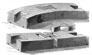
The bricks may be made either square or curved and of any size. They are well adapted for constructing vaulting, each being formed to suit the shape of the arch and provided with a number of mortises proportionate to its size. The circular pieces may be used with advantage in the building of lighthouse or other towers. The Chronique de l'Industrie, to which we are indebted for our facts, says that the method has been used in France to considerable extent and with excellent results.
