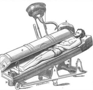
upper part for a hight of about 12 inches. In the upper to prevent escape of heated air at the top of the bath. E, cistern fcr shower bath. F, pillow, with hinged head board to turn up when the bath is not in use. G, rack and pinion for raising or lowering the bath to the level of a bed, for use of an invalid. H, heating apparatus.
