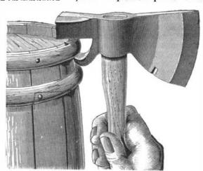
sists, simply, in a claw, made upon the hammer end of an ordinary hatchet, which serves to grasp the top hoop of a barrel. By the aid of the handle as a lever and the hatchet head as a fulcrum, the hoop can be quickly removed uninjured, thus allowing the head of the barrel to be easily taken out. Patented Nov. 12, 1872, by Mr. D. E. Weaver, of Cheviot, Ohio.
