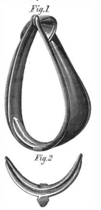
ty, Dr. Edward Batwell, of Ypsilanti, Michigan, has recen ly patented, April 15, 1873, a metal plate which extends up some distance, and thus prevents the collar from closing on the horse's shoulder. The form of the device, which may be made of any suitable metal, together with its mode of application are readily understood from the annexed illustra-
