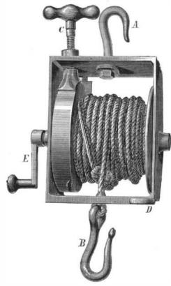
sling being hung to the other hook. The operator then grasps the handle, D, with the left hand, and the screw, C, with the righthand, and thus regulates his downward movement. By tightening the screw, a slow descent may be effected by means of the crank, E. The invention is stated to be cheap, efficient, and not liable to get out of order. For further particulars regarding agencies, sale, etc., address the patentees, Messrs. Merritt & Sweetser, P. O. Box 2,643, North Bridgwater, Mass.
