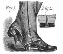
Dr. Batwell states that the invention has been fully tested, d a diameter to fit within a flange on a metal plate and to pro ject below the same, forming a wearing surface of the heel. This is attached by a fastening screw and a conical metal washer formed to fit the under side of the screw head. The latter is forced into the disk, which it pushes into the dovetail flange by which it is securely held. As the wearer turns upon his heel, the plate will partially revolve and change its
