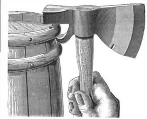
sists, simply, in a claw, made upon the hammer end of an or dinary hatchet, which serves to grasp the top hoop of a barrel. By the aid of the handle as a lever and the hatchet head as a fulcrum, the hoop can be quickly removed uninjured, thus allowing the head of the barrel to be easily taken out: Patented Nov. 12, 1872, by Mr. D. E. Weaver, of Cheviot, Ohio.
